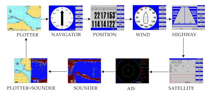
Press the [MODE] key to choose a display mode. Each time the key is pressed, the display mode changes in the sequence shown above.
